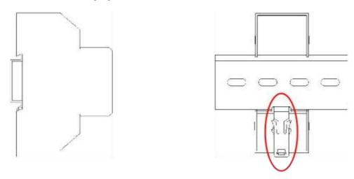
4) the installation of the guide rail has been completed.
